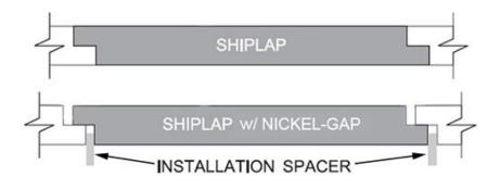
**PRO TIP:** Use a spacer (such as a nickel) to maintain a consistent gap between the Shiplap Planks when installing with a gap.
