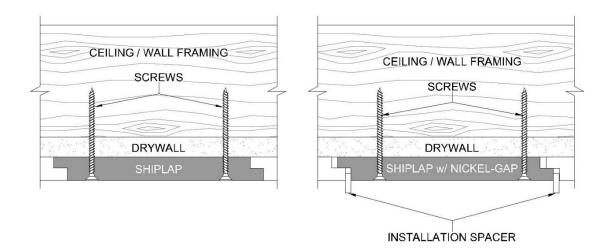
Face nailing and/or screwing of traditional lap-joint type Shiplap Planks is a necessary and acceptable practice.
