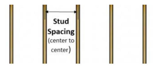
Once you have identified the on-center joist or stud spacing, your Shiplap Planks will need to be cut to lengths which conform to that spacing to ensure that the end-to-end seams (aka butt-joints) land centered on a joist or stud and be fastened at each of the joist or stud locations as required for proper installation.
