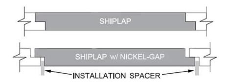
PRO TIP: Use a spacer (such as a nickel) to maintain a consistent gap between the Shiplap Planks when installing with a gap.
