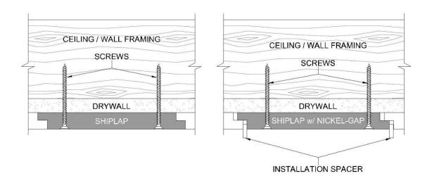
Face nailing and/or screwing of traditional lap-joint type Shiplap Planks is a necessary and acceptable practice.
