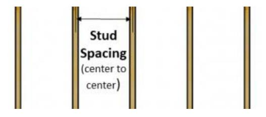
Once you have identified the on-center joist or stud spacing, your Shiplap Planks will need to be cut to lengths which conform to that spacing to ensure that the end-to-end seams (aka butt-joints) land centered on a joist or stud and be fastened at each of the joist or stud locations as required for proper installation.
