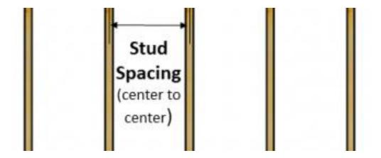
Once you have identified the on-center joist or stud spacing, your Shiplap Planks will need to be cut to lengths which conform to that spacing to ensure that the end-to-end seams (aka butt-joints) land centered on a joist or stud and be fastened at each of the joist or stud locations as required for proper installation.
