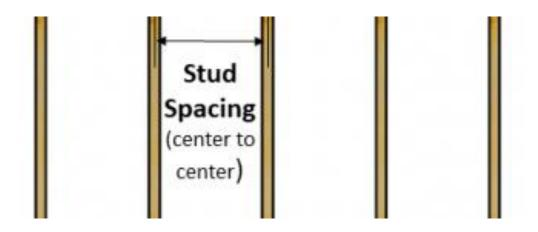
Once you have identified the on-center joist or stud spacing, your T&G Planks will need to be fastened at each of the joist and/or stud locations.
